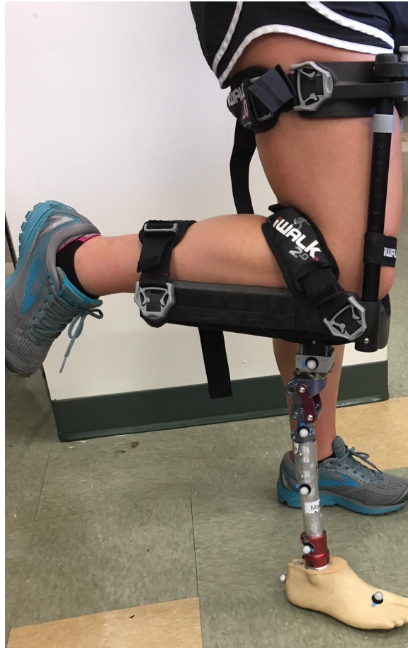
Figure 16: Prosthetic simulator with the SACH foot and reflective markers.
